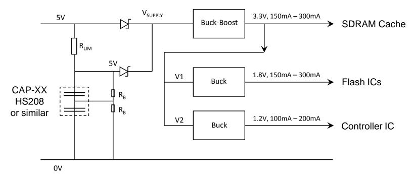
This diagram illustrates a simple design for power backup in an SSD using a supercapacitor.
