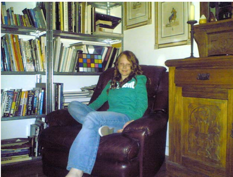
Fig 10: Photo taken in the same conditions as Fig 1 using the same camera phone modified with a supercapacitor to drive 4 x PWF1 LEDs at 0.9A each for a total flash power of 15W. The girl is no longer shadowed and the colours in the colour reference chart beside her are clear compared with Fig 1, which was taken using low power LED flash.
