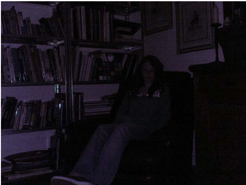
Fig 1: Photo taken in very low ambient light using a low current LED and 1W flash power. The girl is 2m from the camera. Note the colour reference chart beside the girl and how the colours are barely apparent.
