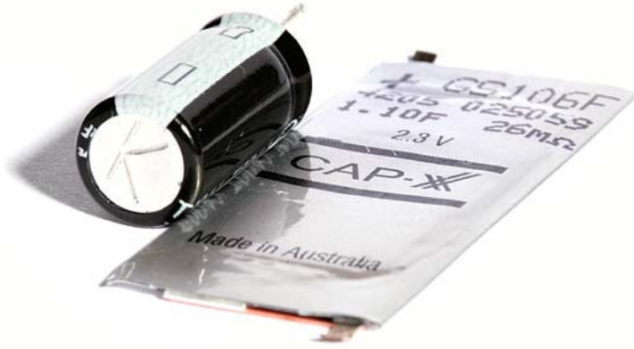
Fig 11: Size comparison between cylindrical electrolytic storage capacitor used for xenon flash and thin prismatic supercapacitor used for LED Flash.
